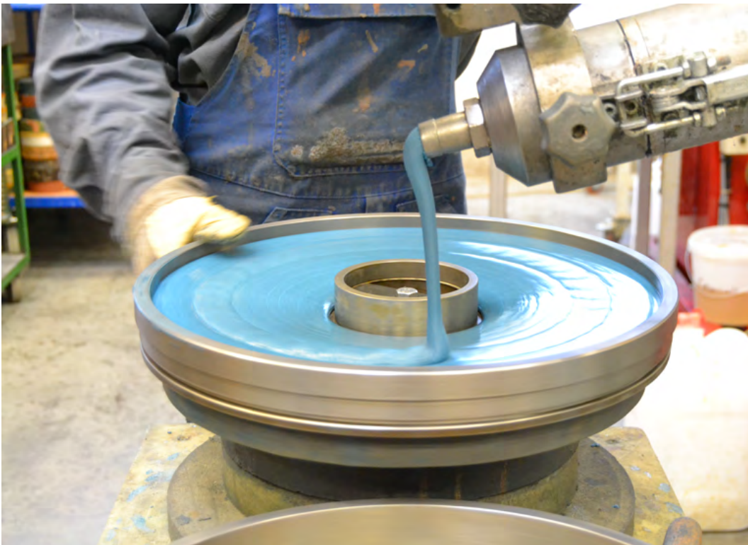
Filling the mixture into the mould
