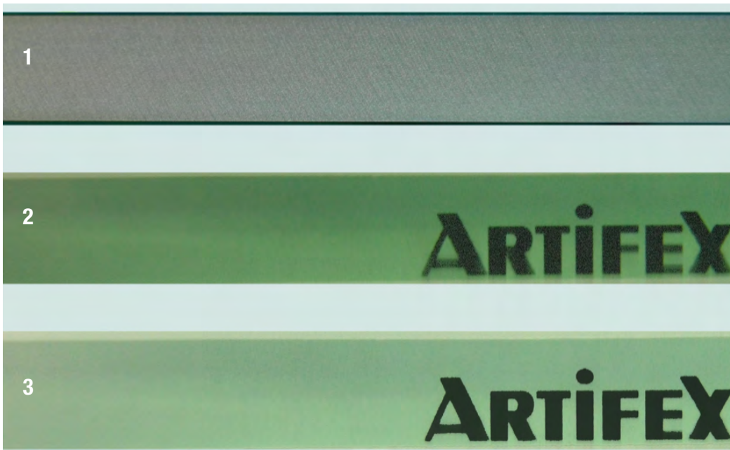
Processed glass edges (1 diamond pre-grinding, 2 pre-polishing, 3 High gloss finishing) (Foto: Artifex)
