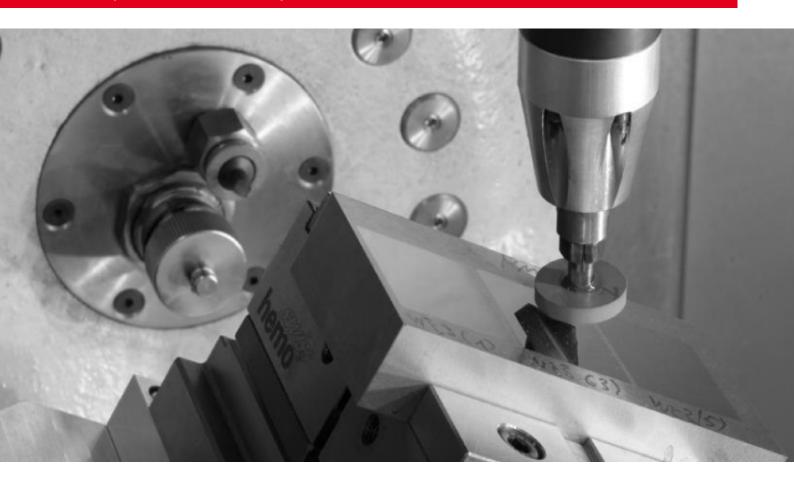
Polishing of hard metal with elastic bonded diamond tools
