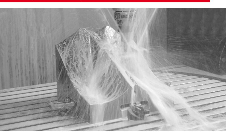
Automated polishing with a CNC machining center in mold making
