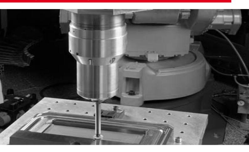
Automated polishing with robots in mold making
