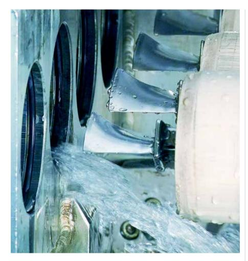
were installed in the casings. Or alternatively, you would have individual airfoils that could be mounted by bracing, or other methods, into segments," Bernd says. "Nowadays, we have technologies in place that allow the manufacture of very precise vane segments out of one single piece of material. Similarly, on the disk side, in the past you had disks and blades separated, but nowadays you can produce it as an integrated part, which is a so-called 'blisk' - a blade and disk combination.
